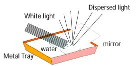
We can place the water tray with mirror inside in sunlight to produce rainbow on the wall.
