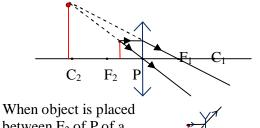
between  $F_2$  of P of a concave lens, the image is formed at the object side between focus and optic centre. The image is virtual,
