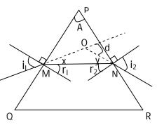
Now fix two pin on the line which was drawn with an angle to the surface 'PQ'. Observe the images at 'PR' side and fix another two pins such that four pins lie along a straight line.
