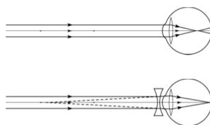
This can be made possible only when a concave lens is used.
