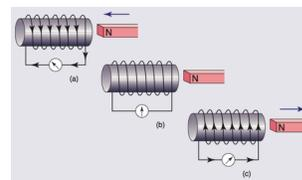
south pole is facing towards the coil, then also the needle deflects. Whenever there is a continuous change of magnetic flux linked with closed coil, the current is generated.
