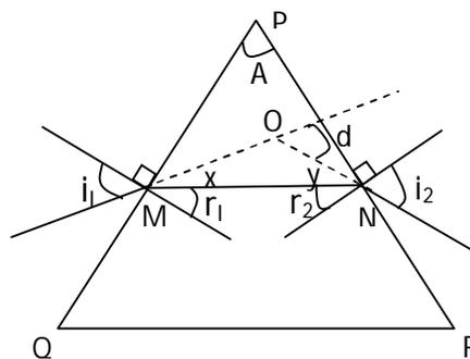
Now fix two pins on the line which was drawn with an angle to the surface 'PQ'. Observe the images at 'PR' side and fix another two pins such that four pins lie along a straight line.
